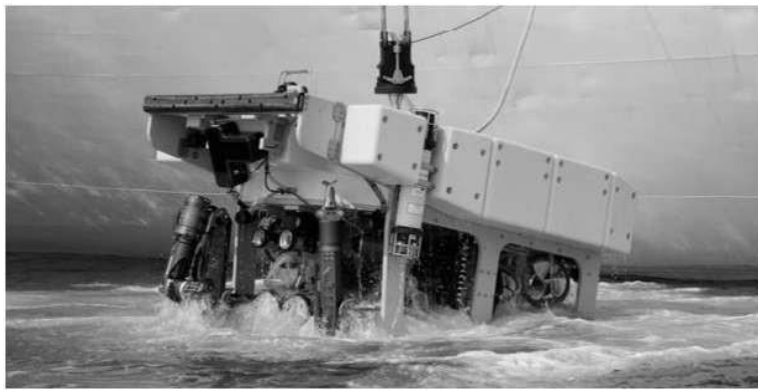
Fig. A remotely operated underwater vehicle (ROV)
